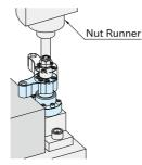
2. Travelling Turn the hex. head with the nut runner and the clamp arm swings to the clamping position.
