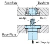
Supply air for unclamping. The wedge goes up and releases the balls.
